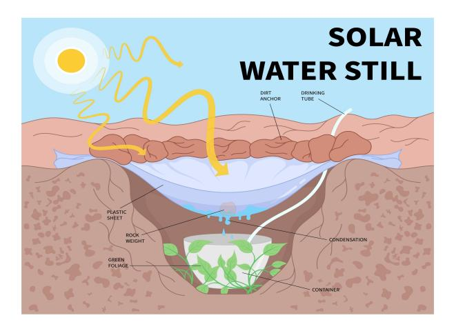
A "solar still" is a simple device that utilises the evaporation condensation technique to convert impure salt water into distilled fresh water by eliminating dissolved salts as well as other dissolved impurities and suspended solids.
